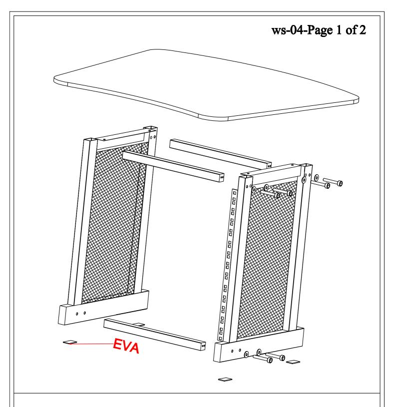
1. Assemble side panels and cross bar supports as shown and tighten bolts firmly. Stick the EVA pads under the bottom of the legs if necessary.
