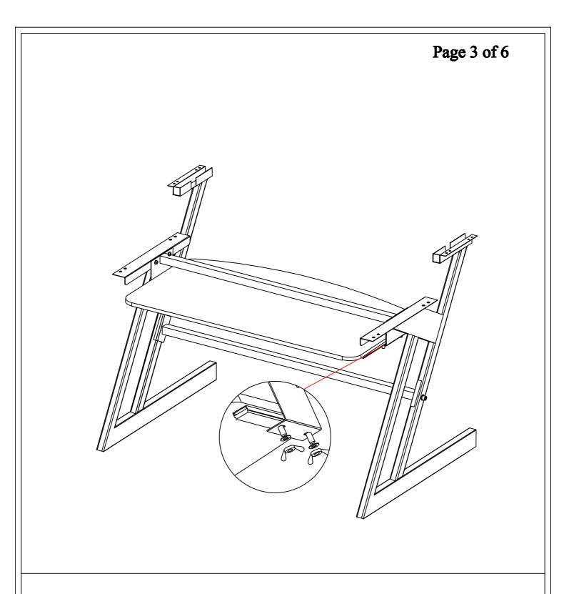
3. Place keyboard shelf in support barckets and bolt in place, tigten nuts till desired shelf pull-out tension is achieved.
