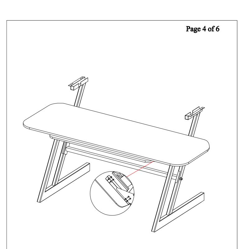
4. Center the main shelf on support brackets and at desired depth, then mount it with provided wood screws.
