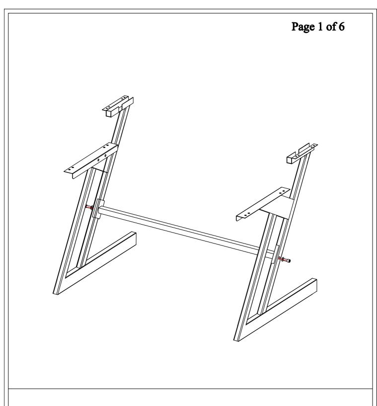
1. Using the allenkey bolts to connect the two main legs with the cross-support bar as the picture showed.
