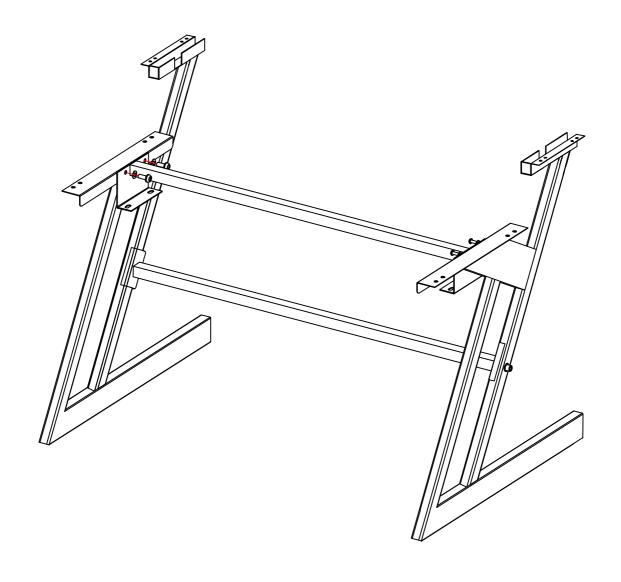
2. Connecting the main shelf cross bracket, and put the keyboard shelf in, then tighten the screws.
